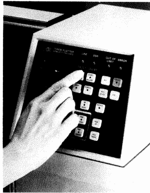
LOWER PINCH WHEELS (STEP 6)
